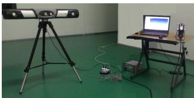
Fig. 2. Laser triangulation 3D scanner
