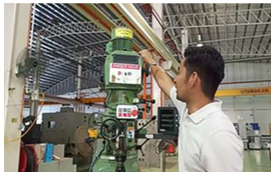
Figure 1.2: User Trying to Unlock the Drawbar by Using a Torque Wrench.
