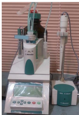
Fig. 5. Total acid number (TAN) test set
