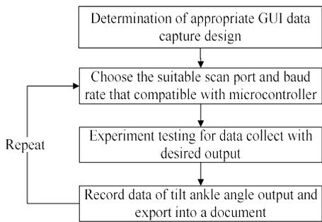
**Figure 9. Design of Overall Graphical User Interface for Data Collection**
