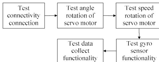
**Figure 11. Test Bench Process to Ensure No Error Occurs**
