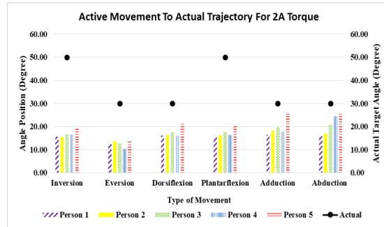
**Figure 15. Active Movement to the Actual Trajectory for low Torque Stiffness Collect Mean Data**
