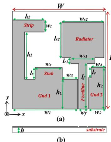
Fig. 1. Geometry of the proposed antenna: a) top view and b) side view.
