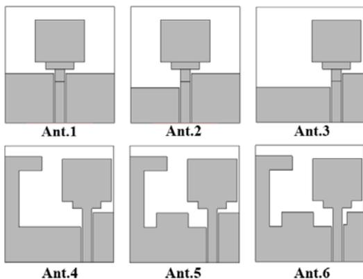
Fig. 2. Six improved prototypes of the proposed antenna
