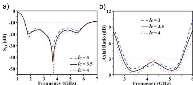
Fig. 6. Effect of  $l_c$  on proposed antenna performances: a)  $S_{11}$  and b) AR
