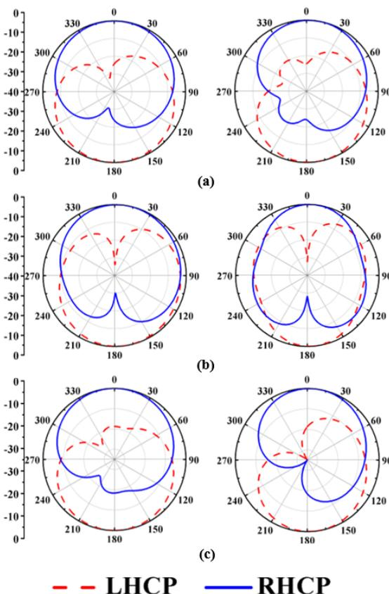
Fig. 8. Simulated radiation patterns at (a) 3.5, (b) 4.5, and (c) 5.2 GHz
