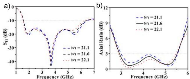
Fig. 4. Effect of  $w_1$  on the proposed antenna performance: a)  $S_{11}$  and b) AR
