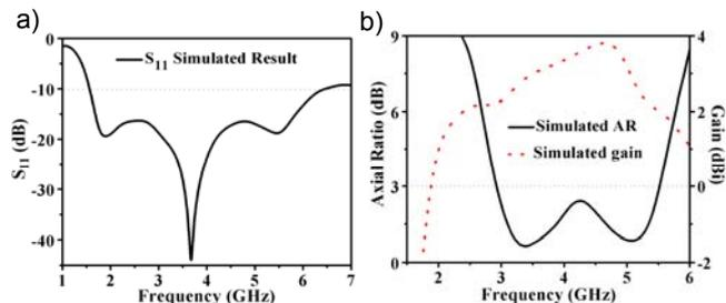
Fig. 7. Simulated results of the designed antenna: (a)  $S_{11}$ , (b) AR, and gain
