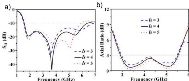
Fig. 5. Effect of  $l_s$  on proposed antenna performances: a)  $S_{11}$  and b) AR
