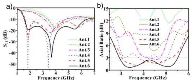
Fig. 3. Simulated results from Ant. 1 to Ant. 6: a)  $S_{11}$  and b) AR
