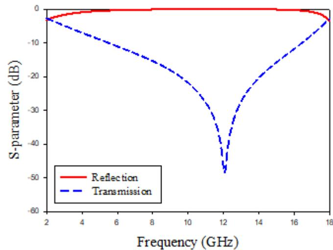
**Figure 6.** Transmission and reflection of FSS at 12 GHz.
