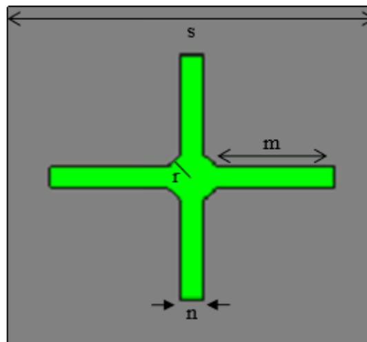
**Figure 2.** Dimension of AMC structure designed at 12 GHz.
