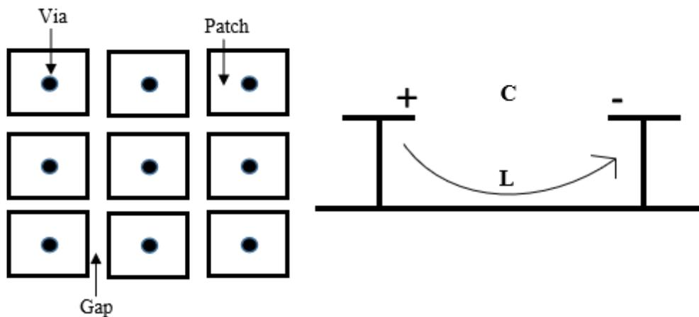
**Figure 1.** Basic AMC structure.
