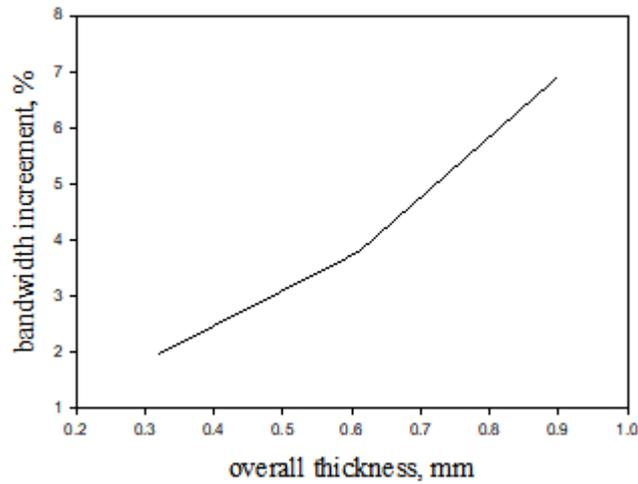
**Figure 8.** Relationship between bandwidth and total structure thickness.
