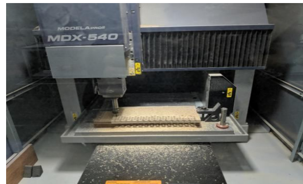
Figure 2: Fabrication of hexagonal cell wood core with CNC gantry router MDX-540
