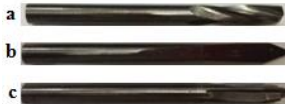
Figure 2: Drill Bits a) Twist Drill, b) Dagger Drill, c) Straight Flute Drill.
