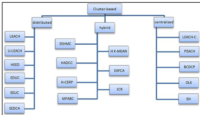
Figure 5: Clustering methods in cluster-based routing protocol
