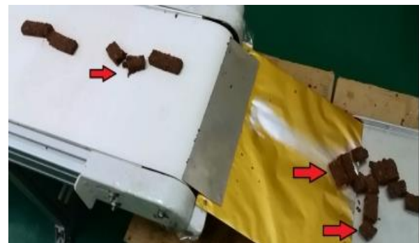
Fig. 2 Breaking snack on a conveyor and pick up tray
