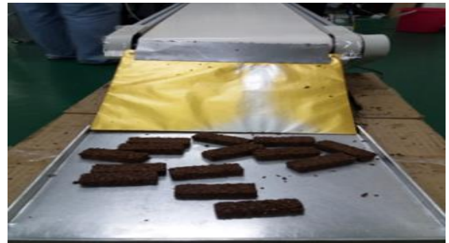
Fig. 11 No broken snack bar on collecting tray
