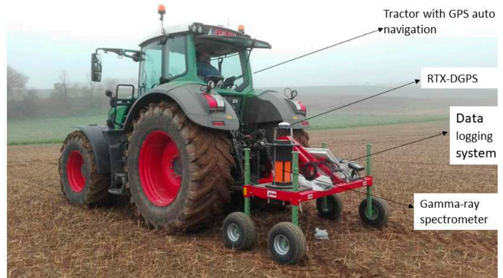
Figure 2. Measurement setup using a portable gamma-ray spectrometer attached to a tractor.
