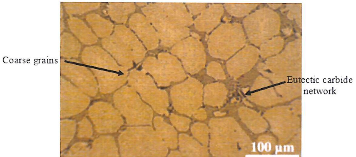
Figure 1.1: An optical micrograph showing the distribution of eutectic carbides of AISI D2 steel alloy in annealed condition (Hamidzadeh, 2013)
