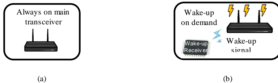
Figure 1. WSN, (a) Without wake-up receiver and, (b) With wake-up receiver
