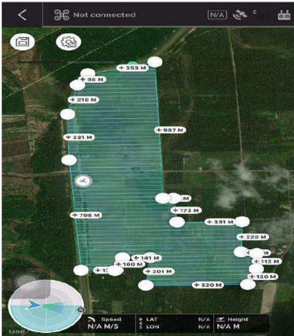
Fig. 3 Waypoint planned by using DJI GS Pro software for 175 acres
