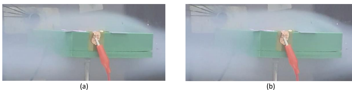
Fig. 5. Temperature image of DBD plasma actuator at (a) velocity 10 m/s, (b) 14 m/s
