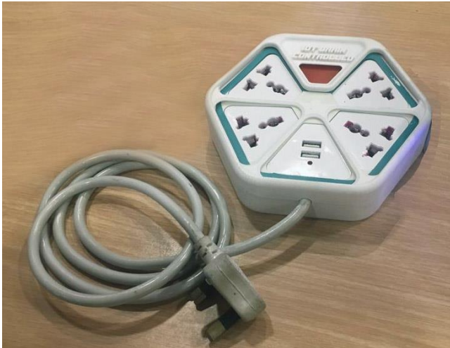
Figure 9. The 3D-printed prototype with the electronic system parts neatly hidden inside.
