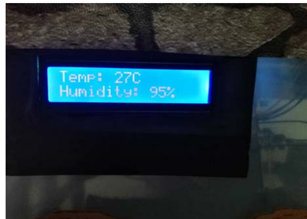
Figure-3. I2C 16 x 2 LCD display temperature and humidity value.
