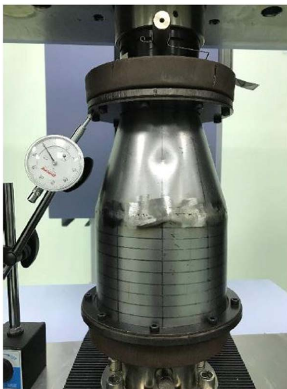
Figure 2. Typical photograph of cone-cylinder specimen testing arrangement using SHIMADZU universal Testing Machine.
