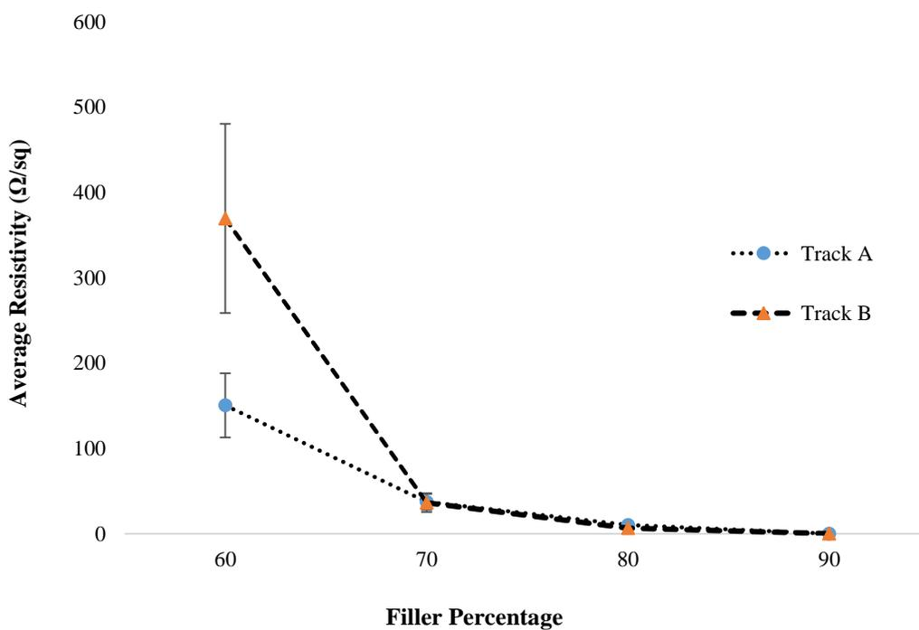
Figure 2: Average sheet resistivity vs filler percentage.
