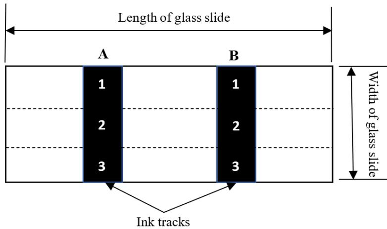
**Figure 1: Printed ink tracks on the glass slide substrate.**
