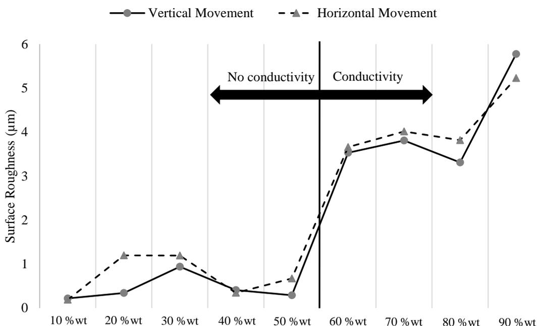
**Figure 5: Surface roughness at different filler loadings for horizontal and vertical directions of measurement.**
