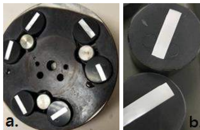
Fig. 3. Grinding of mounted samples; (a) Fixture of the automatic grinder; (b) Mounted samples
