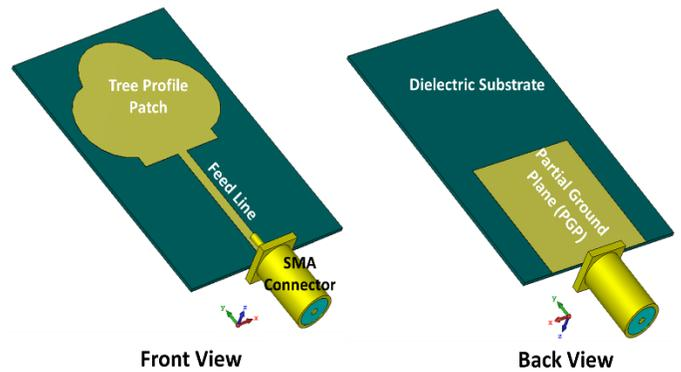
Fig. 2. The Geometry of the Proposed Antenna.
