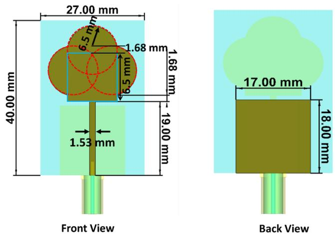
Fig. 3. The Exact Dimensions of the Proposed Antenna.
