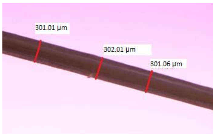
Fig. 3. Optical microscopy image of the Cymbopogon citratus fiber
