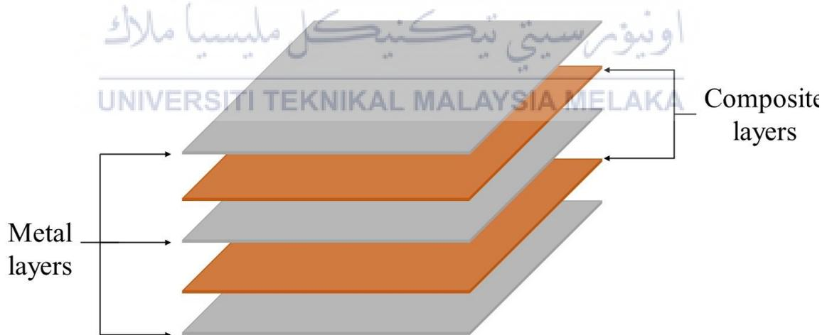
Figure 1.1: A sample lay-up of FML
