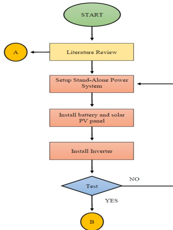
**Figure-1.** Flow chart for installing the stand-alone PV system.
