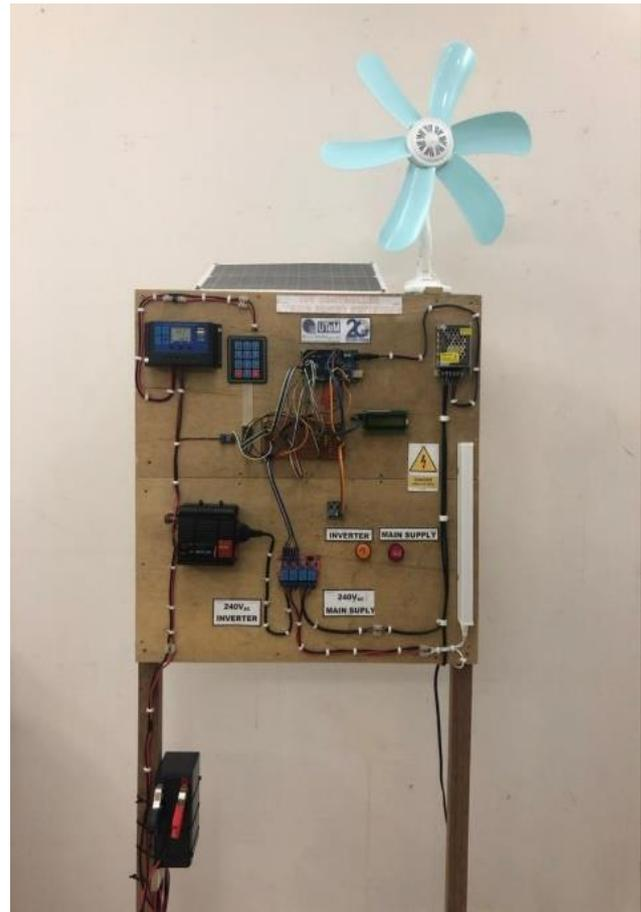
Figure-8. Hardware development of IoT controlled hybrid power switching.
