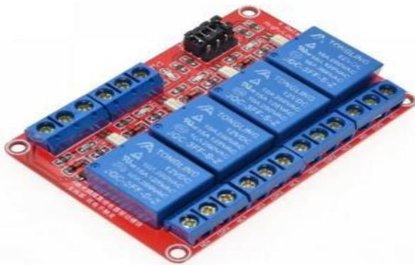
Figure-7. 4-Channel 5V relay module.
