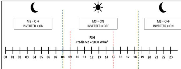
**Figure-10.** Timeline to guide user in controlling the switching timing for manual mode.
