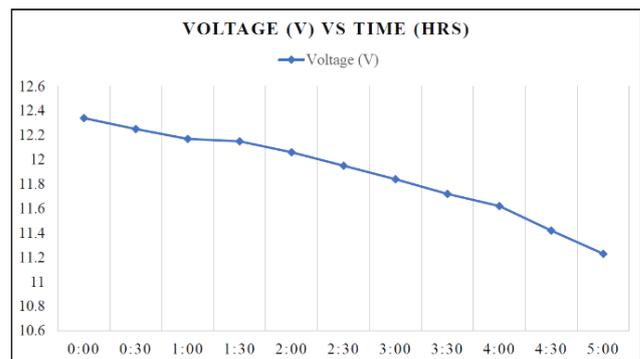
**Figure-12.** Depletion of battery voltage capacity against discharge time in hours.
