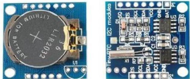
Figure-5. Real-Time Clock (RTC) 1307 module.
