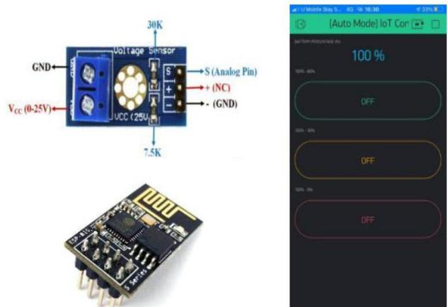
Figure-6. Voltage sensor, ESP8266 Wi-Fi module.
