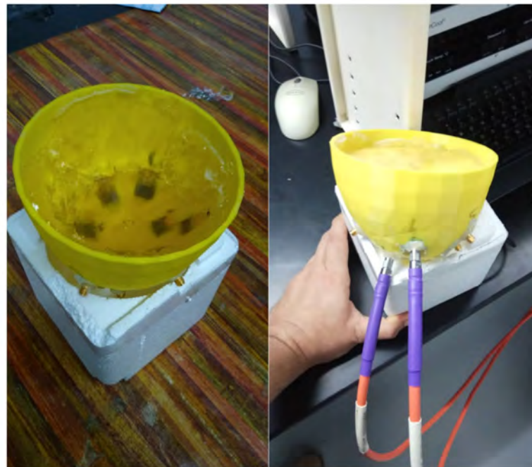
Figure 13. Measurement setup of the breast and the skin.
