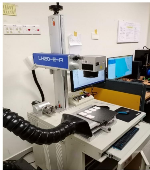
Figure 1. Fiber LH20-E-A Laser engraving machine.
