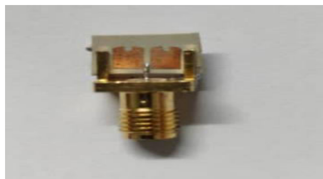
Figure-6. Manufactured single microstrip patch antenna.
