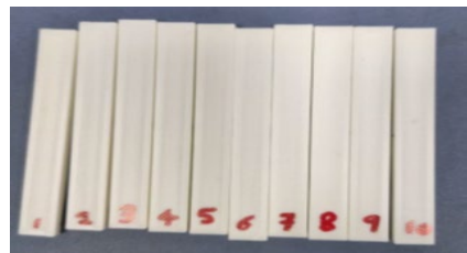
Figure 4: Printed test specimens of ABS material
