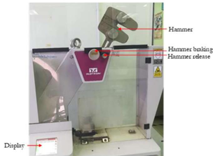
*Fig. 2 Charpy Impact Test Machine (INSTRON CEAST 9050)*
