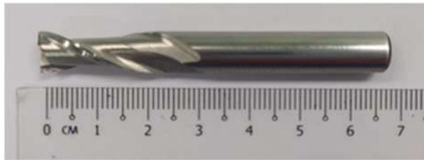
**Fig.7** End mill tool bit
