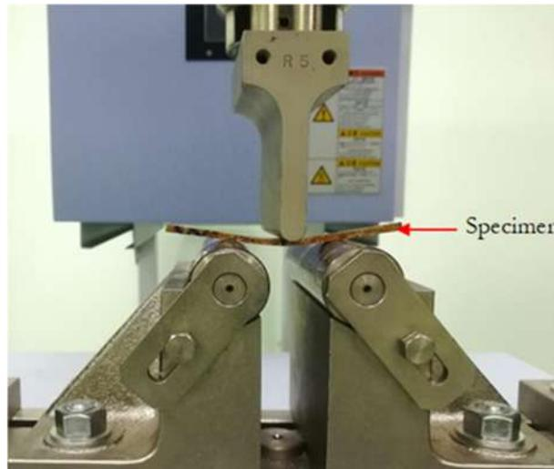
*Fig. 4 Setup of specimen for the flexural test*
