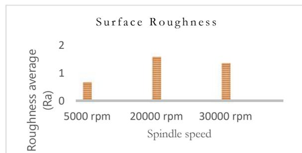
**Fig. 13** Average reading of Ra for pinewood dust at each spindle speed
