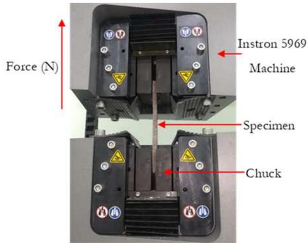
*Fig. 1 Setup of specimens for the tensile strength test*
