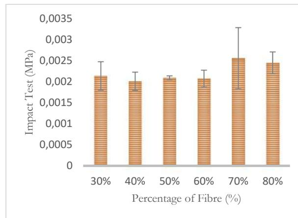
**Fig. 11** Impact strength testing of specimens
