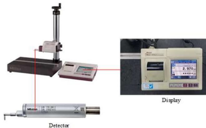
*Fig. 8 Surface roughness machine*
