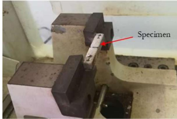
*Fig.3 Setup of specimen for the impact test*
