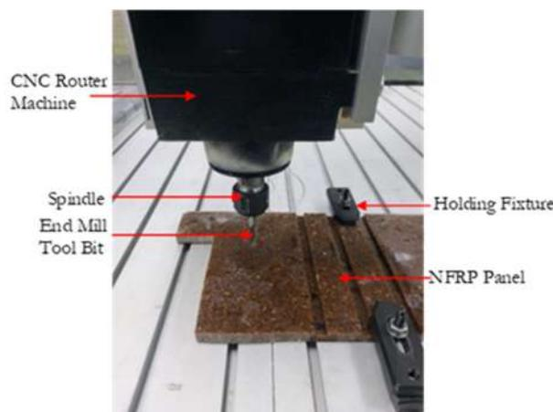
*Fig. 6 CAM-220CNC router machine*
