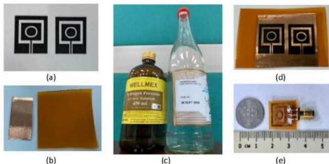
Fig. 16. Prototype Fabrication (a) printed design (b) copper tape and polyimide Kapton film (c) chemical ingredients (d) transferred design (e) final prototype.
