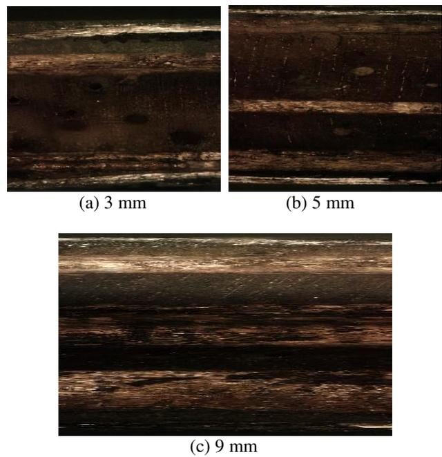
**Figure-6.** Capture image of plywood sandwich laminate composites with 3750 mm/min laser cut machine cutting speed parameters.
