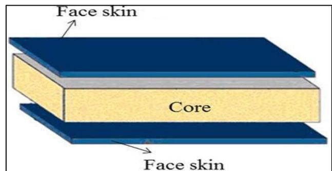
**Figure-2.** Plywood sandwich laminates composite.
