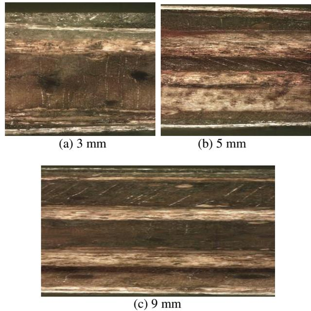
**Figure-5.** Capture image of plywood sandwich laminate composites with 2500 mm/min laser cut machine cutting speed parameters.
