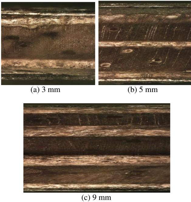
**Figure-4.** Capture image of plywood sandwich laminate composites with 2000 mm/min laser cut machine cutting speed parameters.
