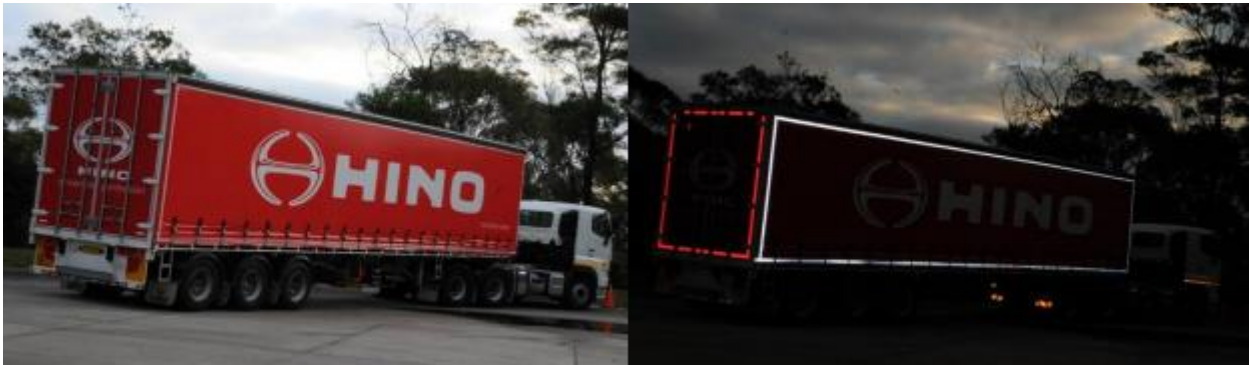
Fig. 1 - The use of reflective strips to enhance heavy vehicle visibility [13]
