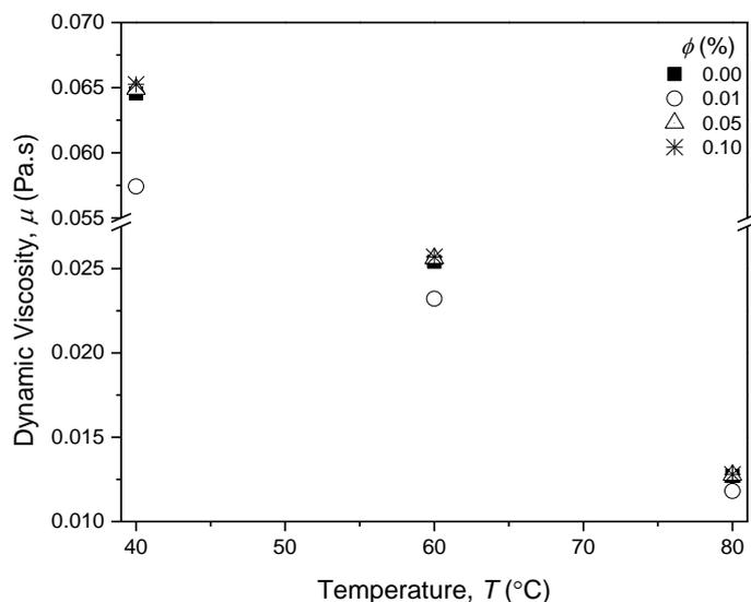
**Fig. 7.** Dynamic viscosity of PVE nanolubricant at various temperature and concentration
