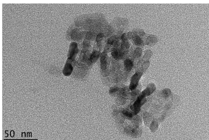
**Fig. 2.** TEM image of  $\text{TiO}_2$ /PVE nanolubricant
