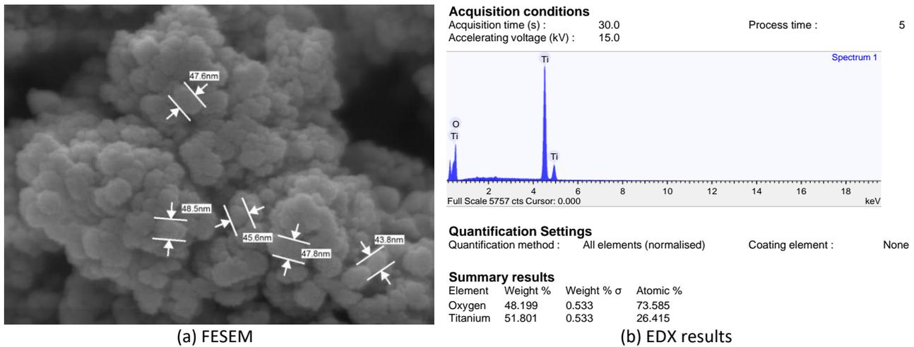
Fig. 3. FESEM-EDX image of TiO<sub>2</sub> nanolubricant
