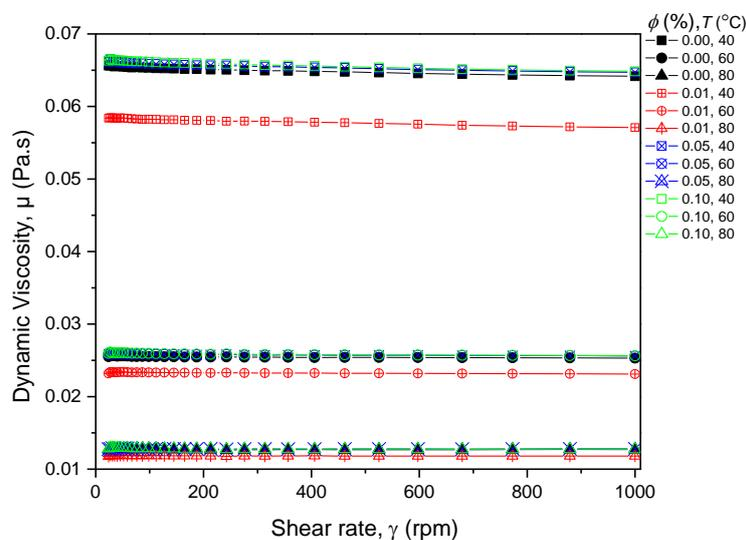
**Fig. 5.** Dynamic viscosity at different shear rate and temperature
