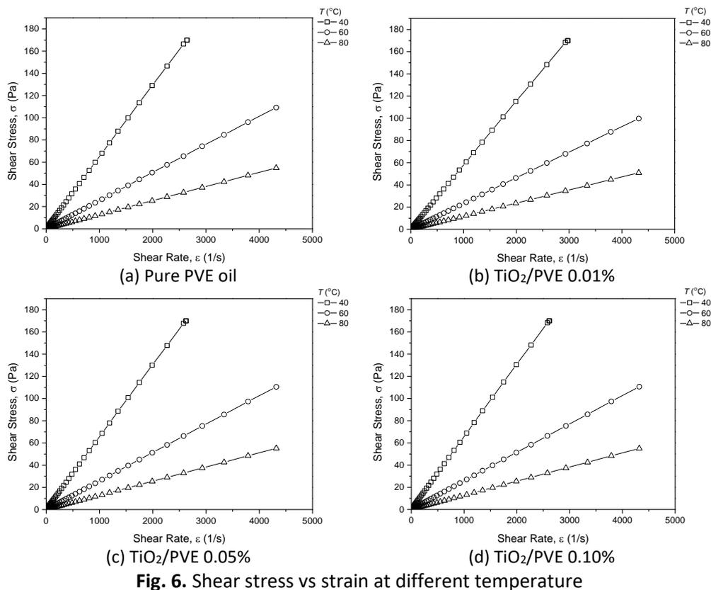
**Fig. 6.** Shear stress vs strain at different temperature
