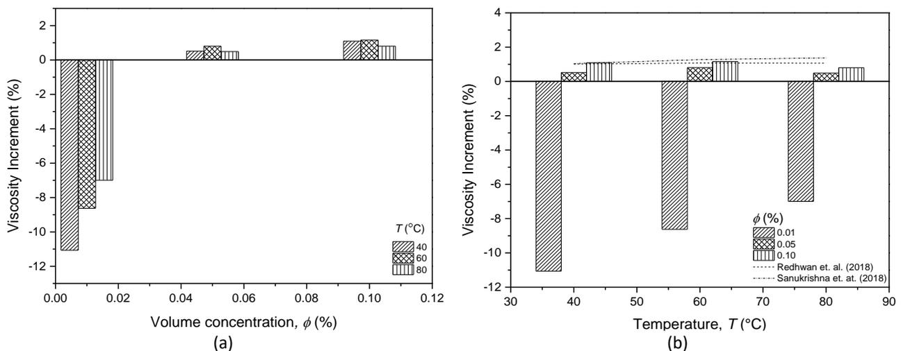
Fig. 8. Viscosity increment of PVE nanolubricant subject to temperature and concentration
