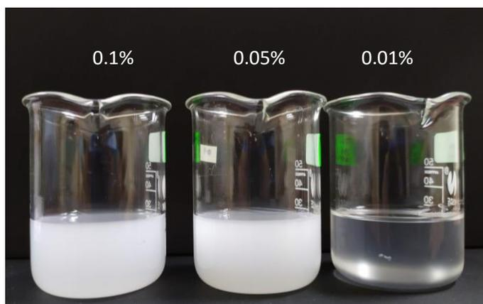
**Fig. 1.** PVE lubricant and prepared  $\text{TiO}_2$ /PVE nanolubricant at different concentration (vol. %)
