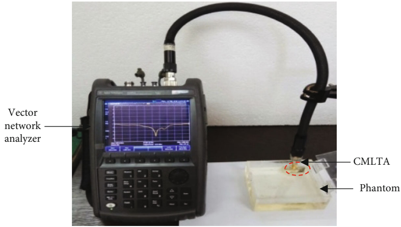
FIGURE 7: Measurement setup of CMLTA in a homogeneous phantom.
