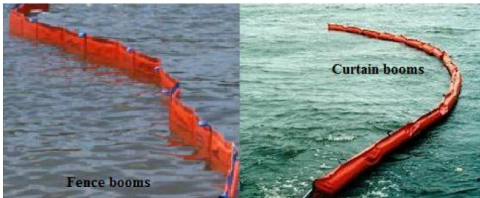
Fig. 2: The types of booms used to control the oil spill spread (Gong et al. 2014).
