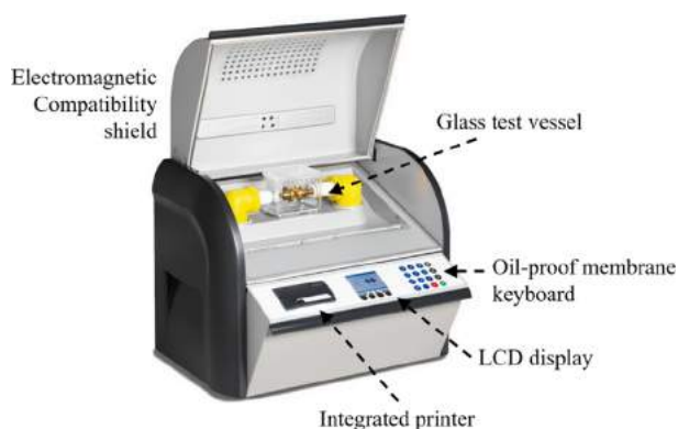
Fig. 4 DTA 100C BAUR oil breakdown voltage tester with 400 ml test vessel in accordance with IEC 60156 standard.
