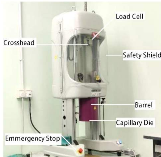
Figure 4. The capillary rheometer used (model Instron SR20).
