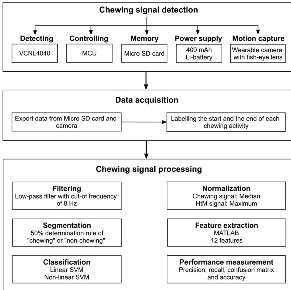
Figure 2. General process flow of automatic chewing detection.
