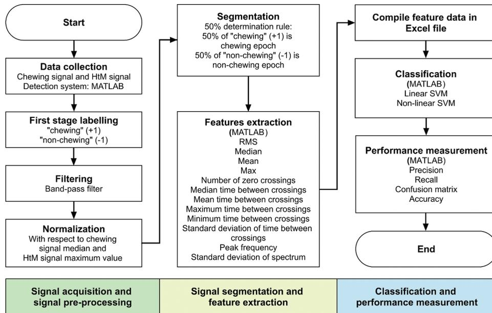
Figure 3. Process flow of chewing signal processing.
