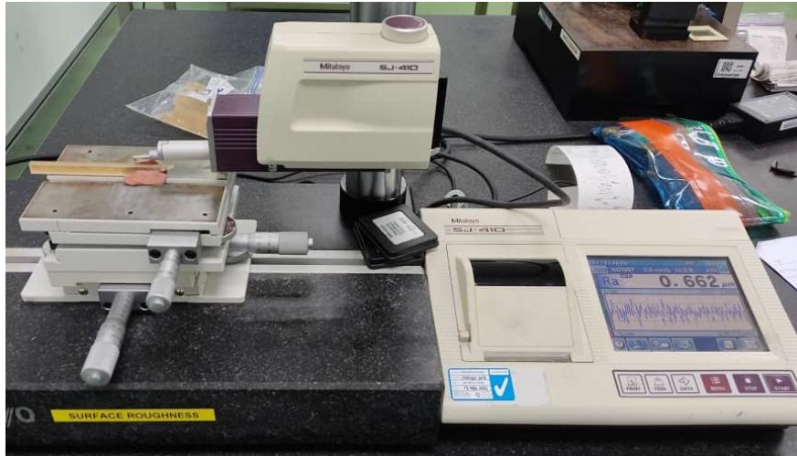
Figure 5. Setup experiment for surface roughness.
