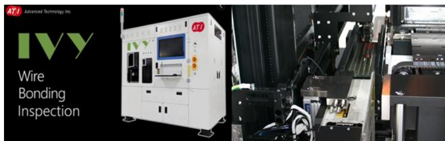
Figure 1.1 Wire Bonding Inspection AOI tool from ADVANCED TECHNOLOGY INC. (ATI) KOREA COMPANY used for strip form inspection
