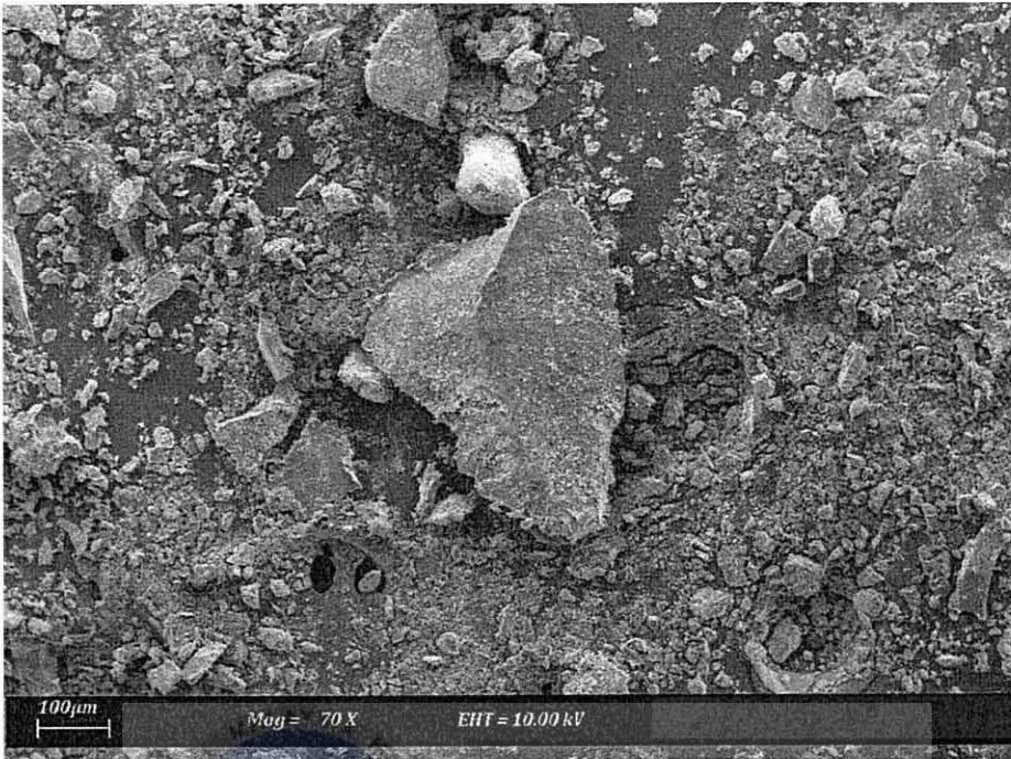
Figure 4.3 (a): Quarry dust particles observed through SEM as received.
