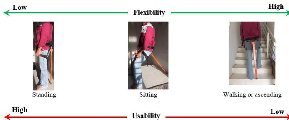
Fig. 3 - Flexibility versus usability of a sit-stand exoskeleton
