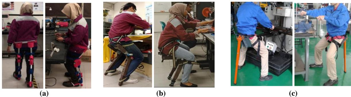
**Fig. 1 - Three prototypes of passive sit-stand exoskeleton developed by authors**
