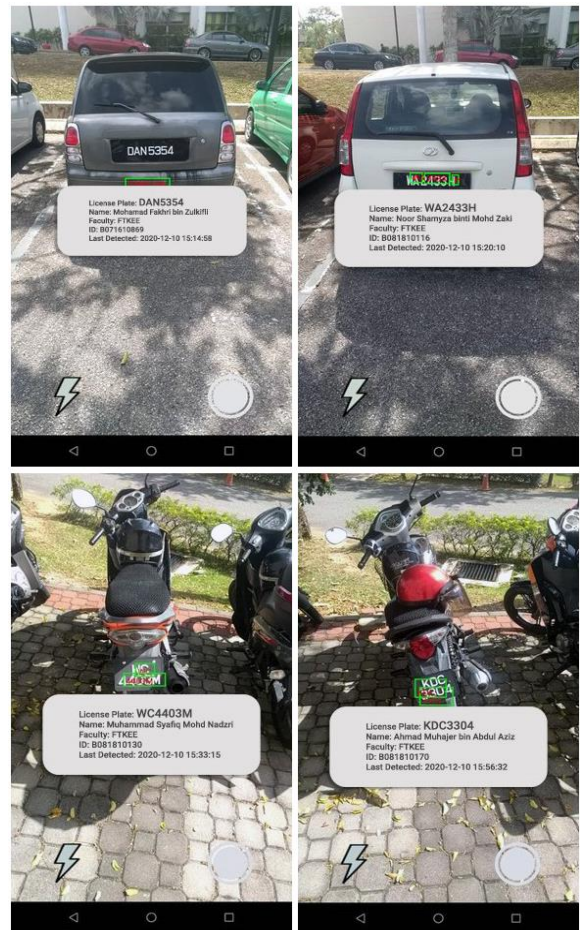
Figure 8 Recognition of license plate numbers that are registered in the database (data label pops up displaying owner identity and details).
