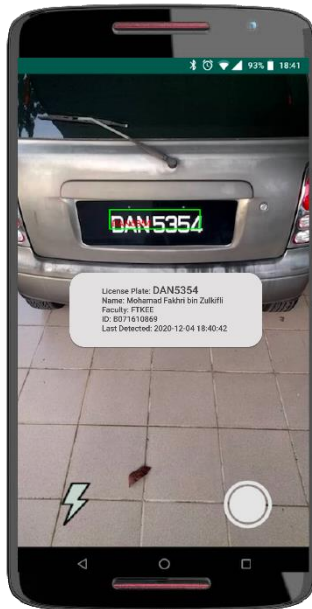
Figure 7 ANPR CNN main app window. Note that the recognition immediately starts once the live-video scanning frame is loaded, and in the event a registered license plate number is recognized, the detailed info label pops up.
