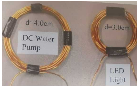
Figure 11. The structure of receiver coils, Rx
