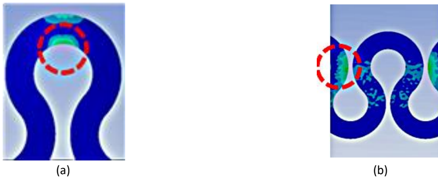
Fig. 6. Simulation of equivalent plastic strain (mm/mm) for horseshoe 45° pattern subjected to (a) longitudinal ( \epsilon_p = 0.073432 ) (b) lateral loading ( \epsilon_p = 0.012903 )
