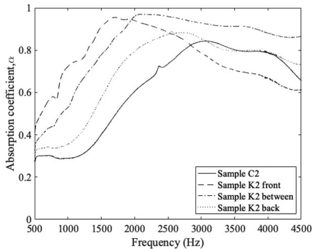
**Figure 8.** Sound absorption performance of coir sample with varied kapok positions.
