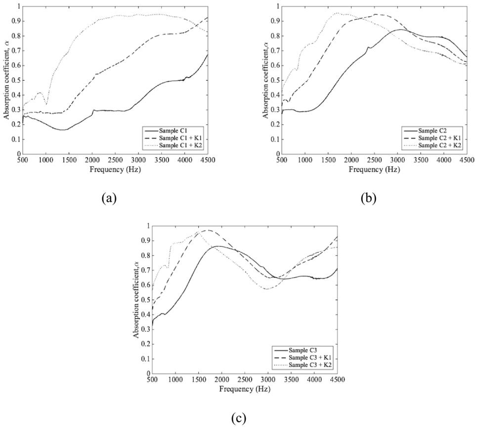
Figure 2. Sound absorption coefficient for coir fiber thickness of (a) 10 mm (C1), (b) 20 mm (C2), and (c) 30 mm (C3) with and without the addition of kapok fibers (Sample K1 and K2).
