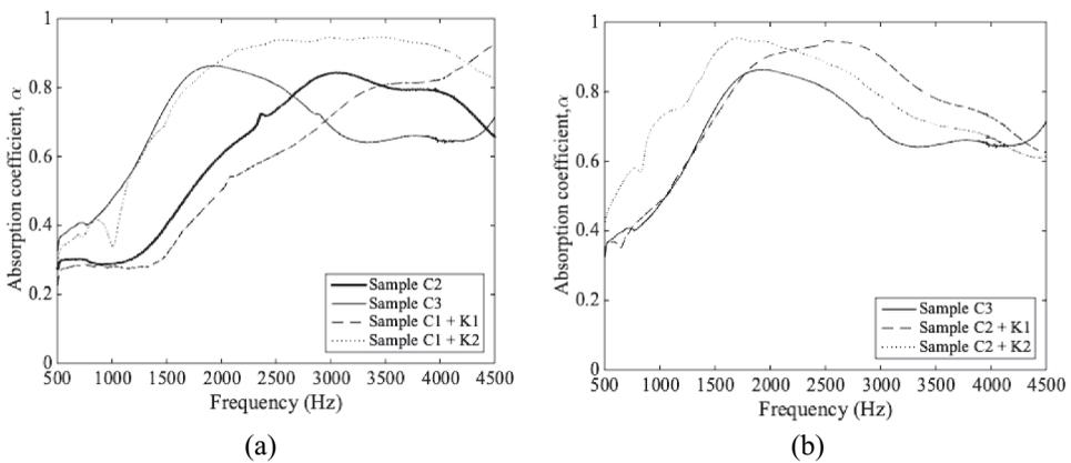
Figure 3. Comparison of coir fiber sound absorption coefficient.
