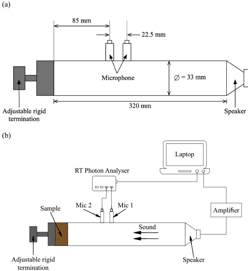
**Figure 1.** (a) impedance tube schematic diagram and (b) impedance tube measurement setup.
