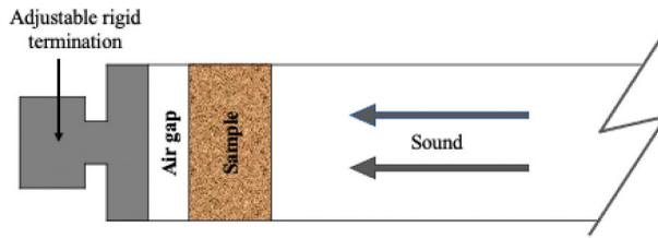
**Figure 4.** Arrangement of sample with the addition of air gap inside the impedance tube.
