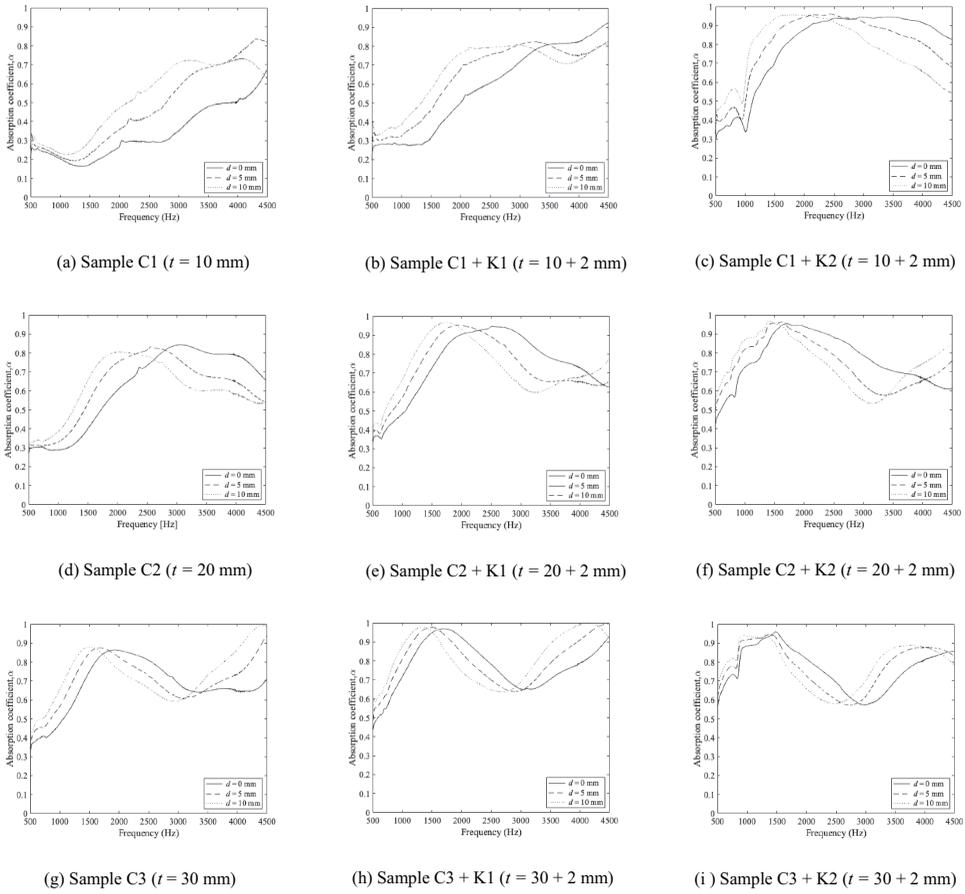
Figure 5. Effect of air gap to the sound absorption coefficient for varied thickness coir with and without the addition of kapok fiber.
