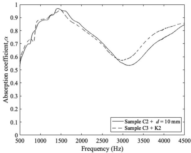
Figure 6. Comparison of sound absorption coefficient for equivalent thickness for the condition of full fiber thickness and fiber added with air gap.
