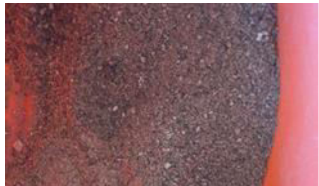
Figure-2. Coconut shell powder after sieved.
