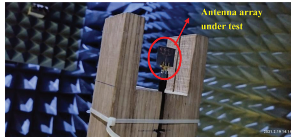
Figure 4: Proposed antenna array under testing
