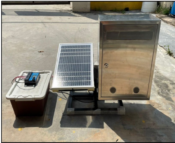
Fig. 7. The Smart Mailbox Notification System with Solar Battery Charging
