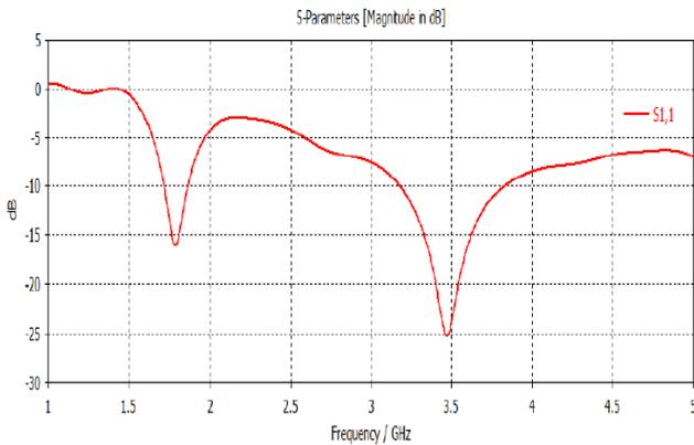
Figure-2. Return loss of the proposed horn antenna.
